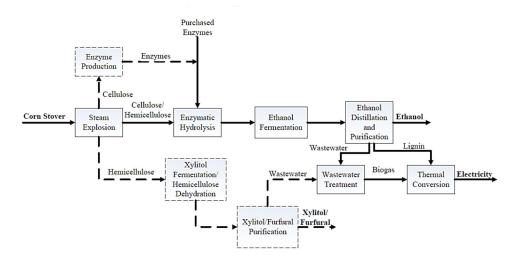
**Figure 10**. General flowsheet of a multi-product lignocellulosic biorefinery producing ethanol and furfural/xylitol (74).
