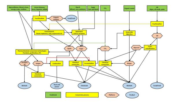
Figure 3.Conversion technologies for biomass based on IEA Bioenergy Task 42 biorefinery<br/>classification system (16)
