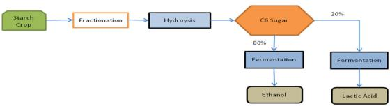
Figure 9. Integrated ethanol and lactic acid production.
