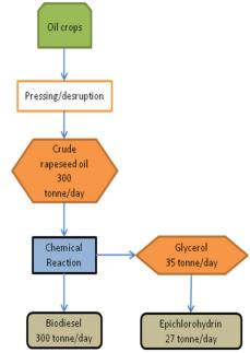
**Figure 11**. Integrated biodiesel and epichlorohydrin production.
