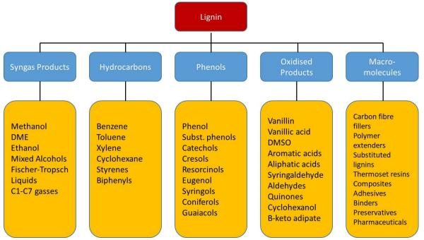
Figure 6. Potential products from lignin (adapted from 46).
